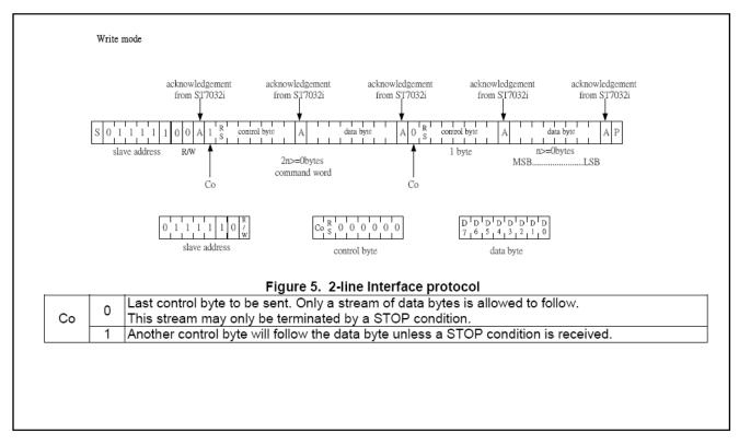
During write operation, two 8-bit registers are used. One is data register (DR), the other is instruction register (IR)
